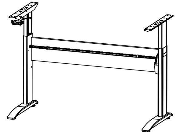
\*\*\* width less than 1060mm is possible to create by cutting down alu tubes connecting the 2 legs
